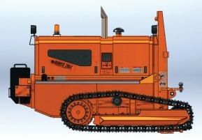
Weight: 7400 lbs. Ground Clearance: 7" Ground Pressure: 4.27 psi.
